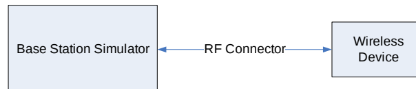
Figure 14-1 Power Measurement Setup
