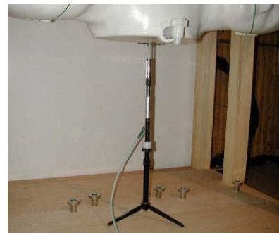
Figure 12-2 System Verification Setup Photo
