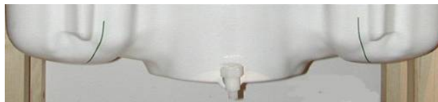
Figure 7-2 SAM Twin Phantom Shell
