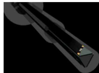
Figure 4-3 Triangular Probe Configuration
