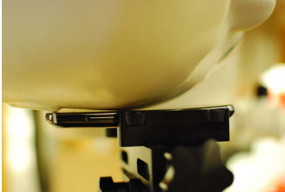
SAR Test Setup Photo 1 – Right Touch
