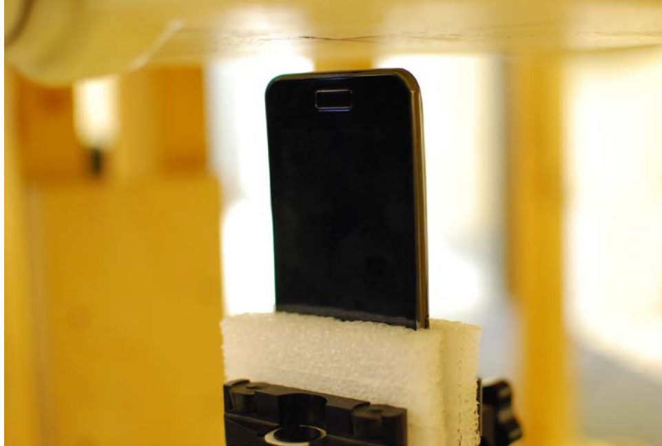
SAR Test Setup Photo 7 – Bottom at 1.0 cm
