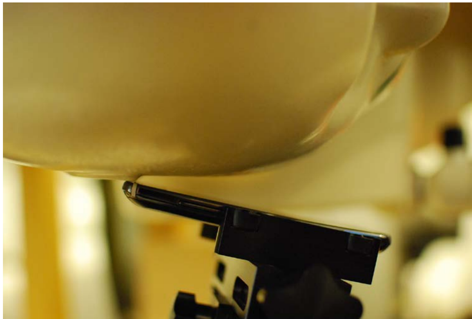
SAR Test Setup Photo 2 – Right Tilt
