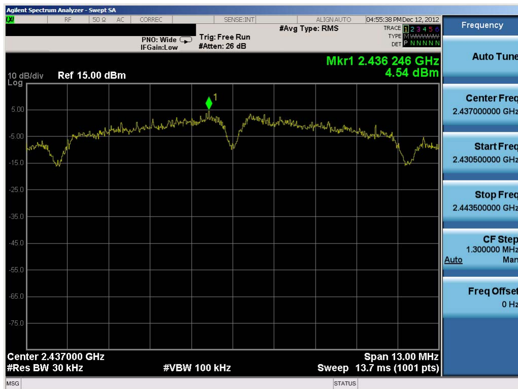
Plot 6-11. Power Spectral Density Plot (802.11b – Ch. 6)
