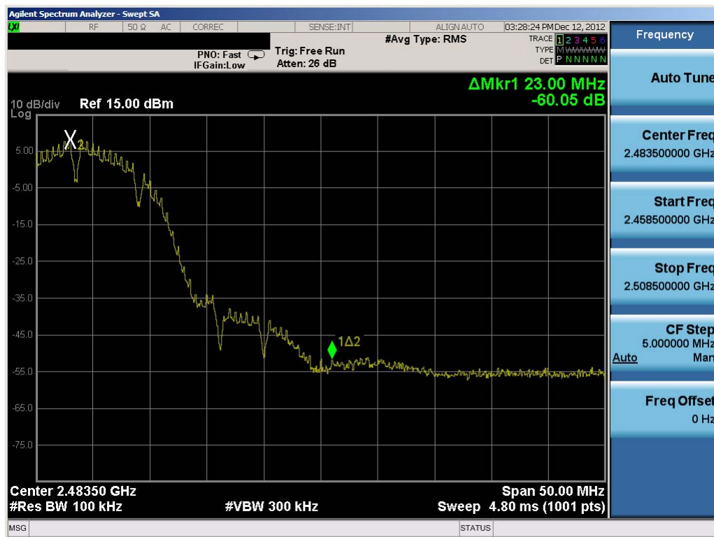
Plot 6-20. Band Edge Plot (802.11b – Ch. 11)
