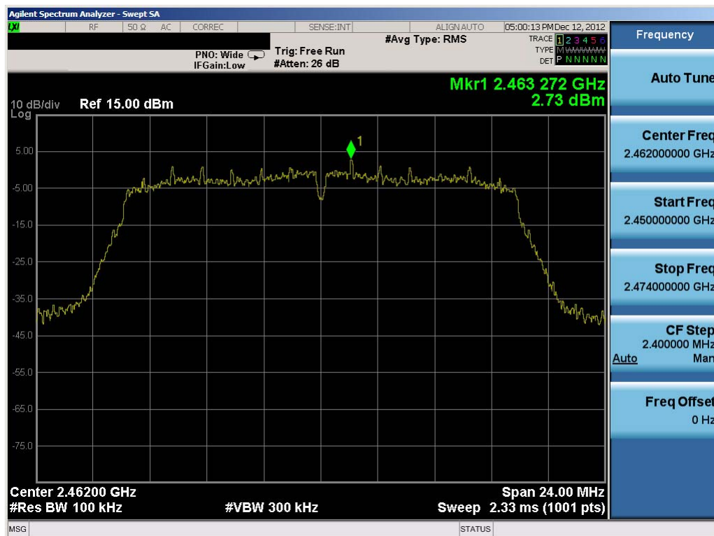
Plot 6-15. Power Spectral Density Plot (802.11g – Ch. 11)
