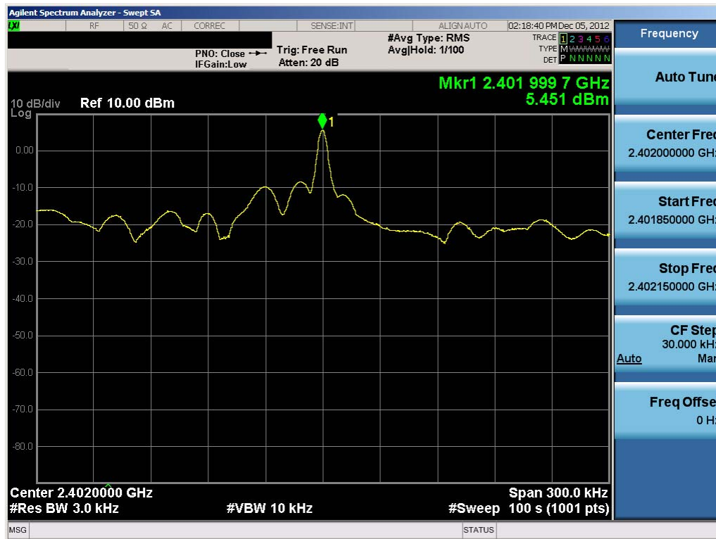
Plot 6-4. Power Spectral Density Plot (Bluetooth (LE) – Ch. 0)
