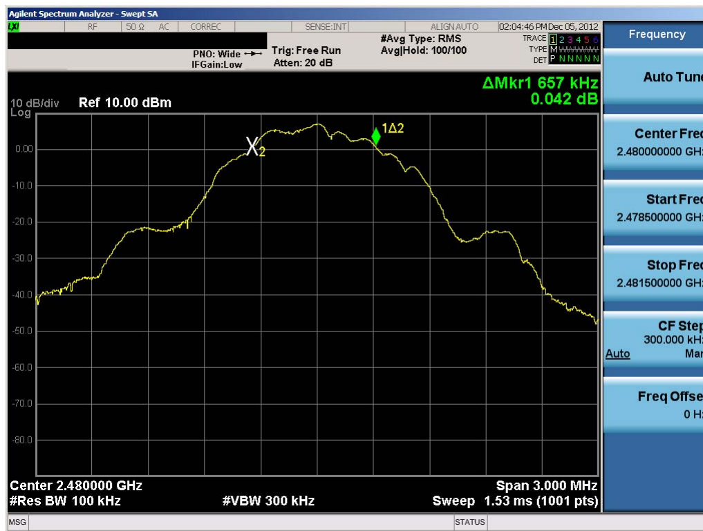
Plot 6-3. 6dB Bandwidth Plot (Bluetooth (LE) – Ch. 39)
