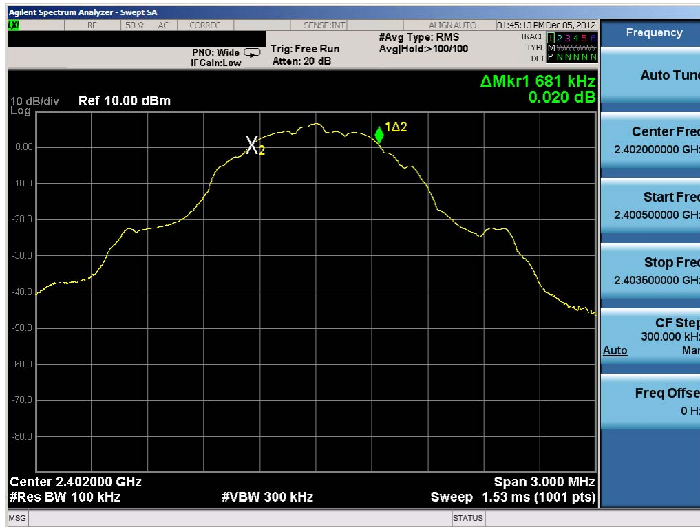
Plot 6-1. 6dB Bandwidth Plot (Bluetooth (LE) – Ch. 0)
