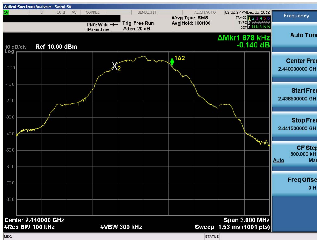
Plot 6-2. 6dB Bandwidth Plot (Bluetooth (LE) – Ch. 19)
