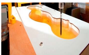
Figure 6-2 SAM Phantom with Simulating Tissue
