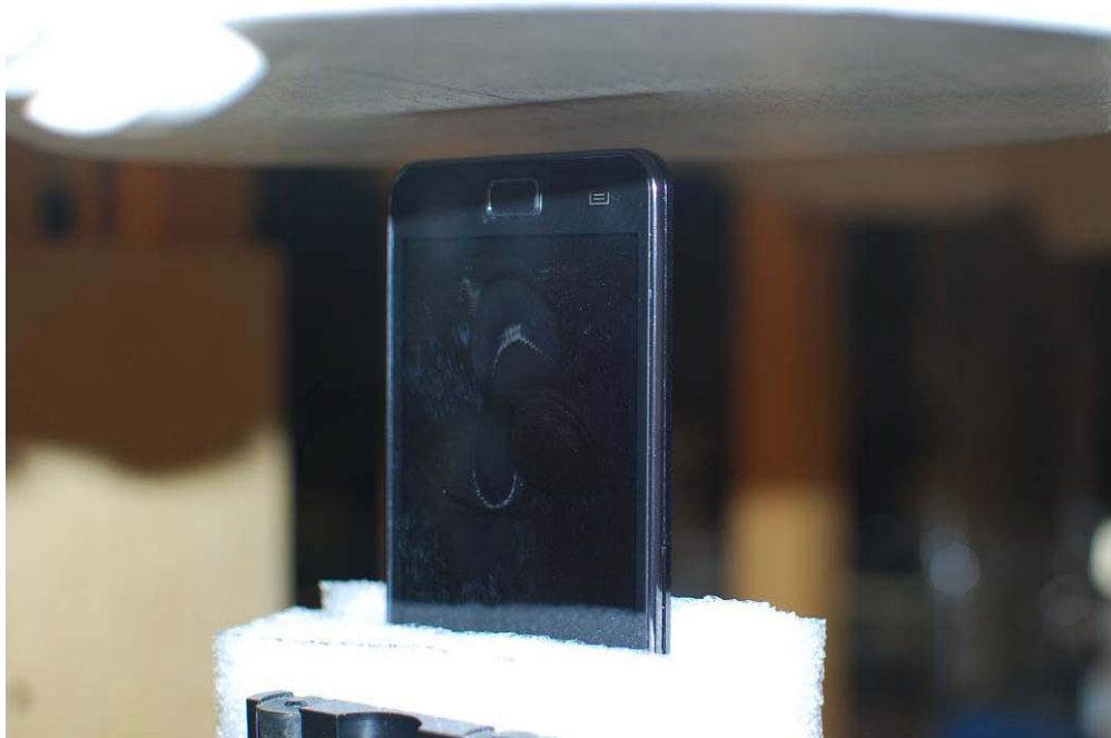
Figure 21-7 SAR Test Photo 7 – Bottom at 1.0 cm
