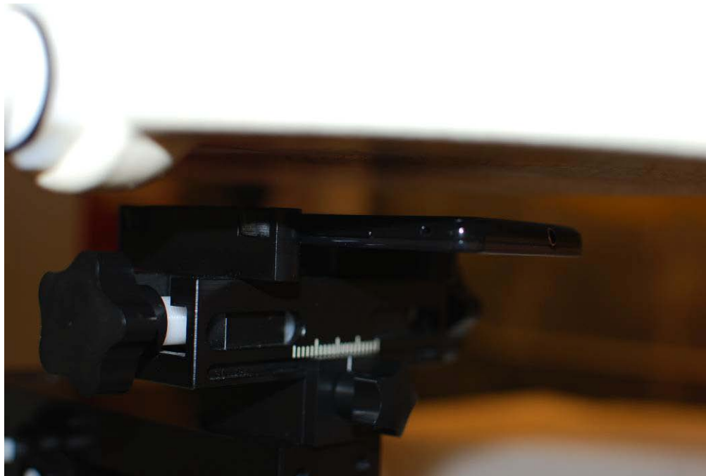
Figure 21-10 SAR Test Photo 10 – Back at 1.5 cm
