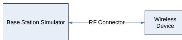
Figure 9-2 Power Measurement Setup
