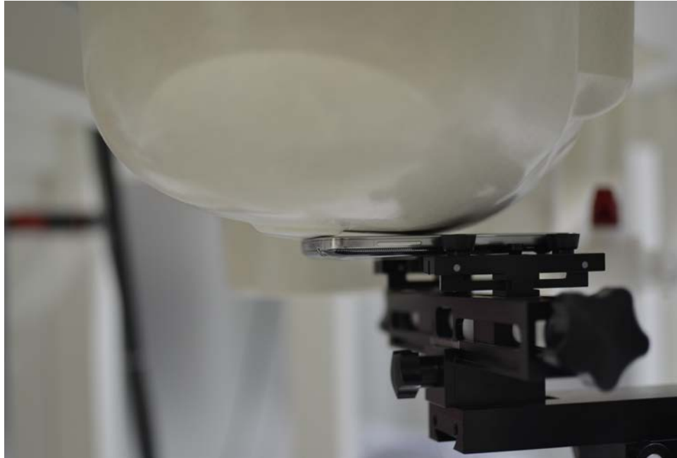
SAR Test Setup Photo 1: Right Cheek
