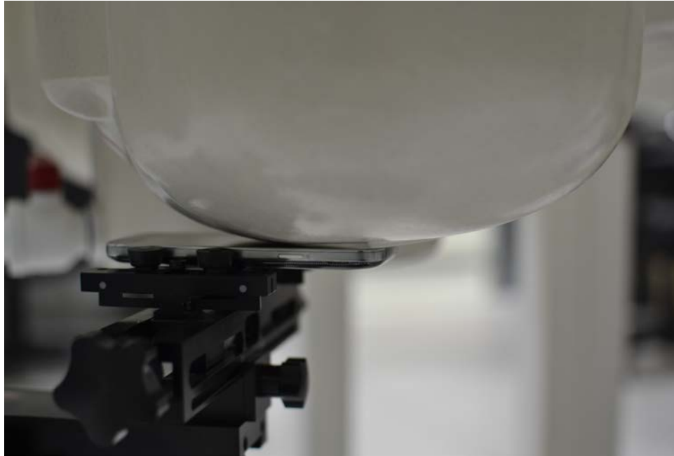
SAR Test Setup Photo 3: Left Cheek
