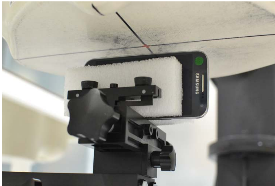
SAR Test Setup Photo 10: Left Edge at 1.0 cm
