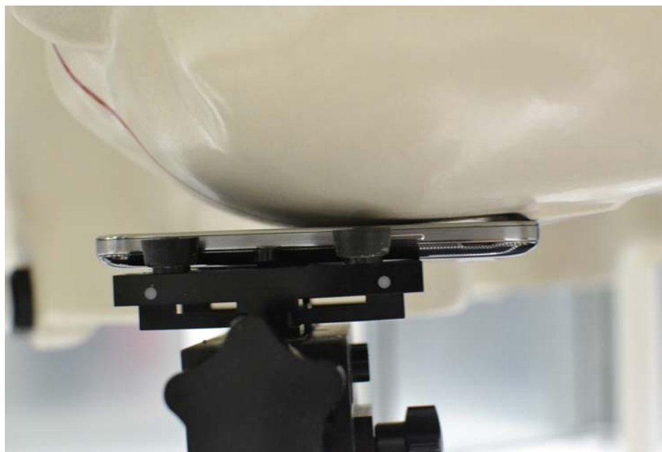
SAR Test Setup Photo 3: Left Cheek
