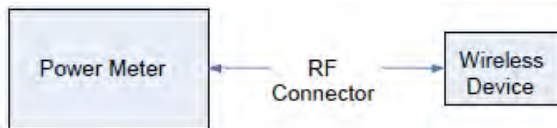
Figure 9-3 Power Measurement Setup
