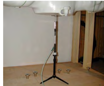
Figure 10-2 System Verification Setup Photo
