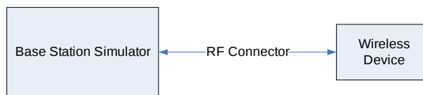
Figure 9-2 Power Measurement Setup
