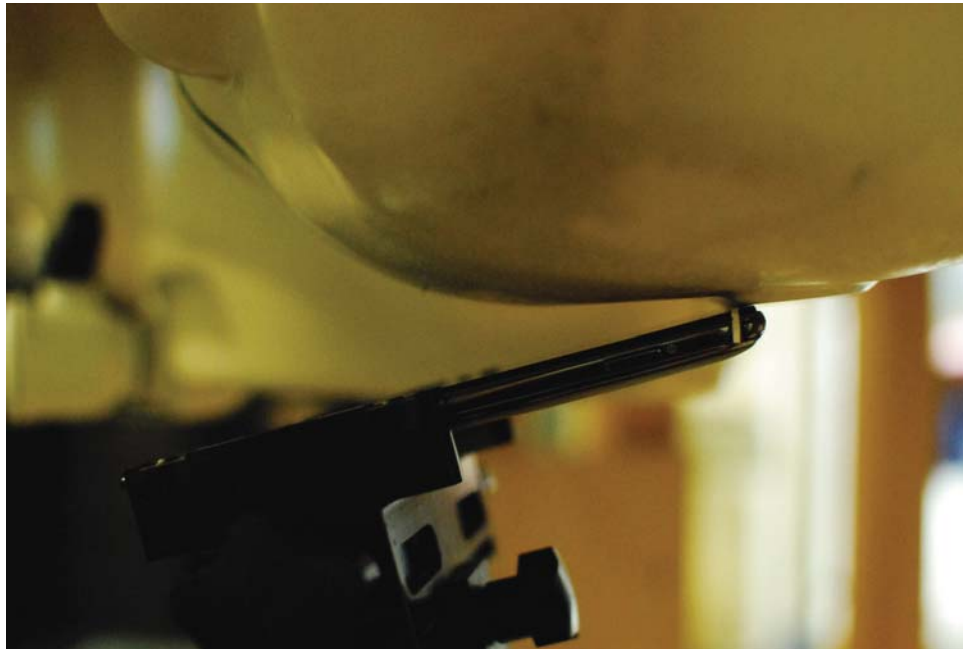
SAR Test Setup Photo 4: Left Tilt
