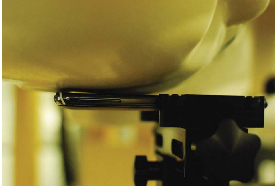
SAR Test Setup Photo 1: Right Touch
