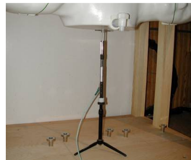
Figure 10-2 System Verification Setup Photo
