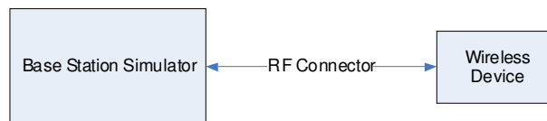
Figure 9-1 Power Measurement Setup
