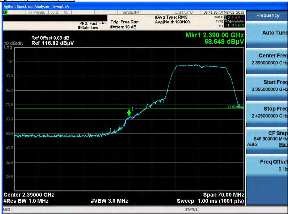
Plot 6-64. Radiated Restricted Lower Band Edge Measurement (Peak)
