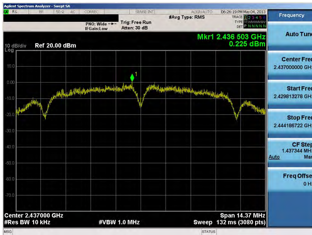
Plot 6-20. Power Spectral Density Plot (802.11b – Ch. 6)
