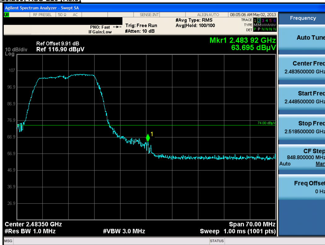
Plot 6-66. Radiated Restricted Upper Band Edge Measurement (Peak)
