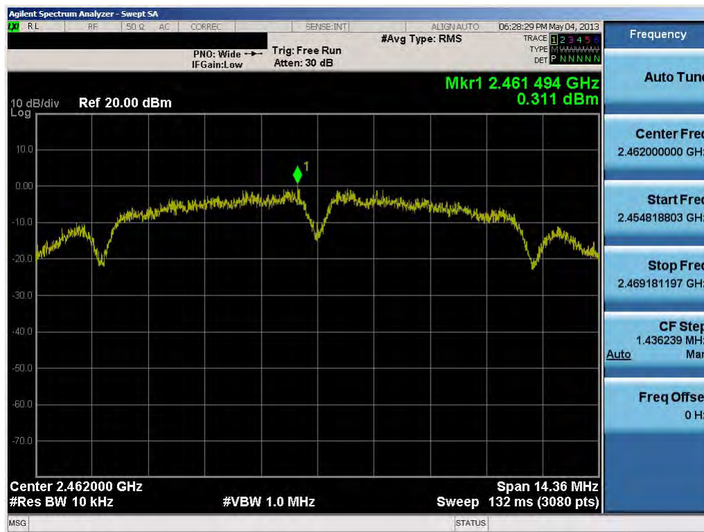
Plot 6-21. Power Spectral Density Plot (802.11b – Ch. 11)
