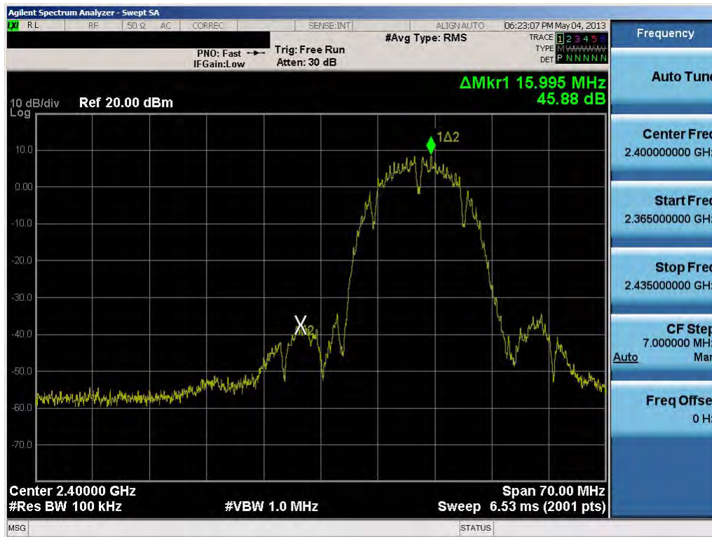
Plot 6-37. Band Edge Plot (802.11b – Ch. 1)
