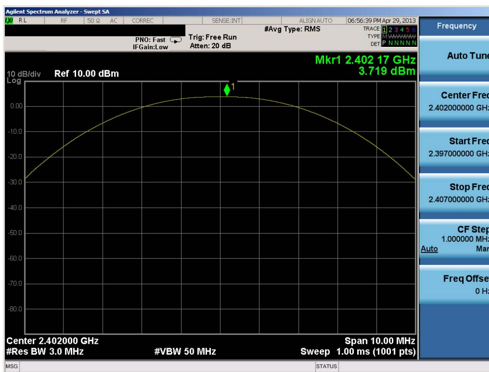
Plot 6-4. Peak Power Plot (Bluetooth (LE) – Ch. 0)
