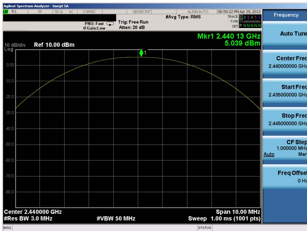
Plot 6-5. Peak Powery Plot (Bluetooth (LE) – Ch. 19)
