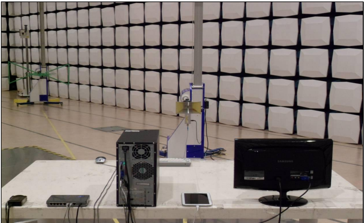
[ Radiated Disturbance for Above 1 GHz – Rear ]
