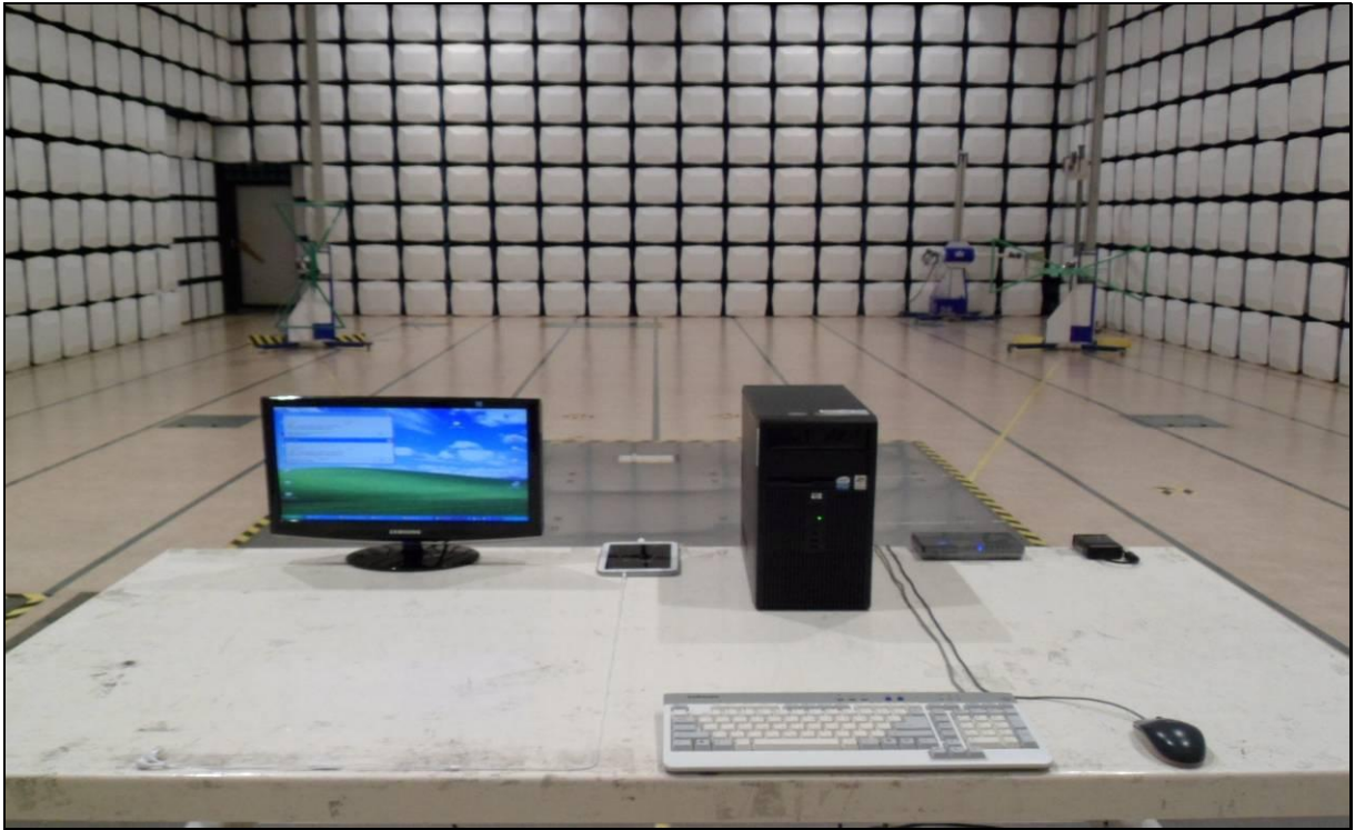
[ Radiated Disturbance for Below 1 GHz – Front ]
