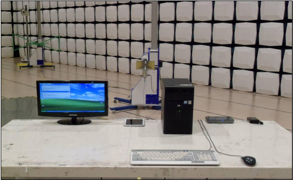
[ Radiated Disturbance for Above 1 GHz – Front ]
