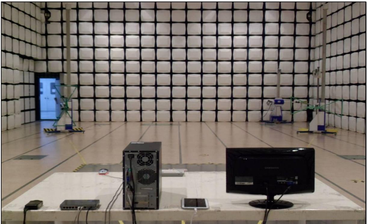
[ Radiated Disturbance for Below 1 GHz – Rear ]
