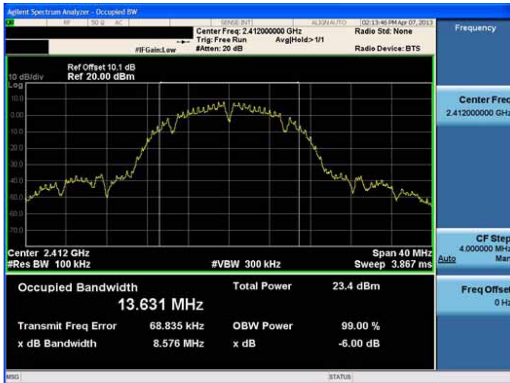
6dB Bandwidth plot (802.11b-CH 6)
