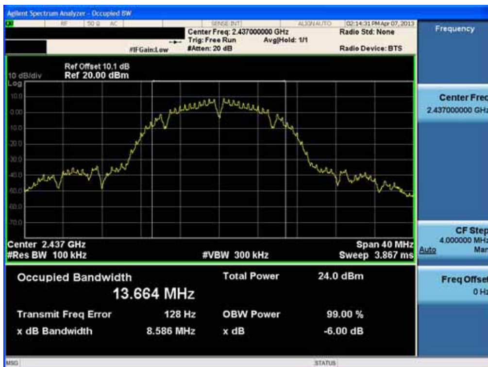
6dB Bandwidth plot (802.11b-CH 6)
