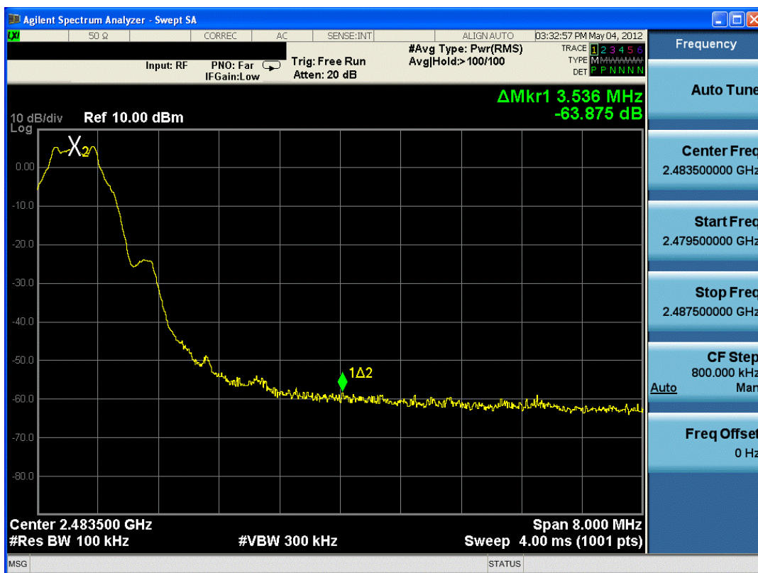
Plot 6-8. Band Edge Plot (Bluetooth (LE) – Ch. 39)
