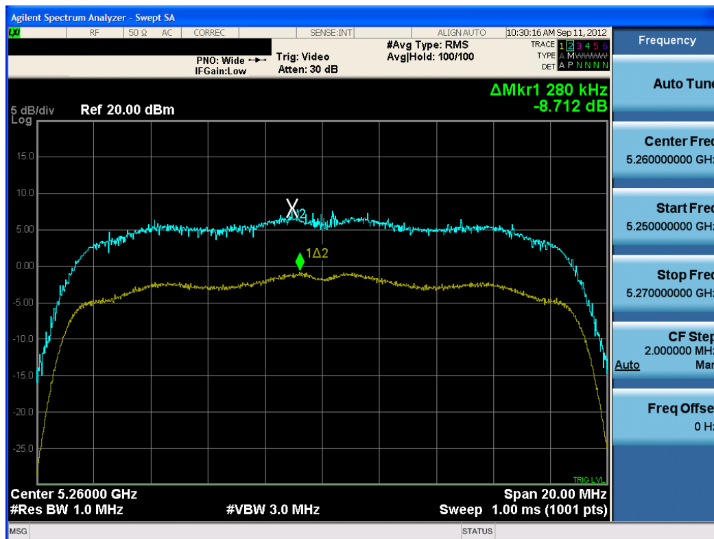
Plot 6-62. Peak Excursion Ratio Plot (20MHz BW 802.11n (UNII Band 2) – Ch. 52)
