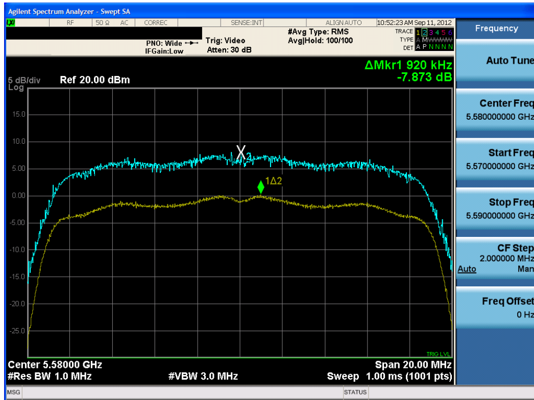
Plot 6-71. Peak Excursion Ratio Plot (20MHz BW 802.11n (UNII Band 3) – Ch. 116)
