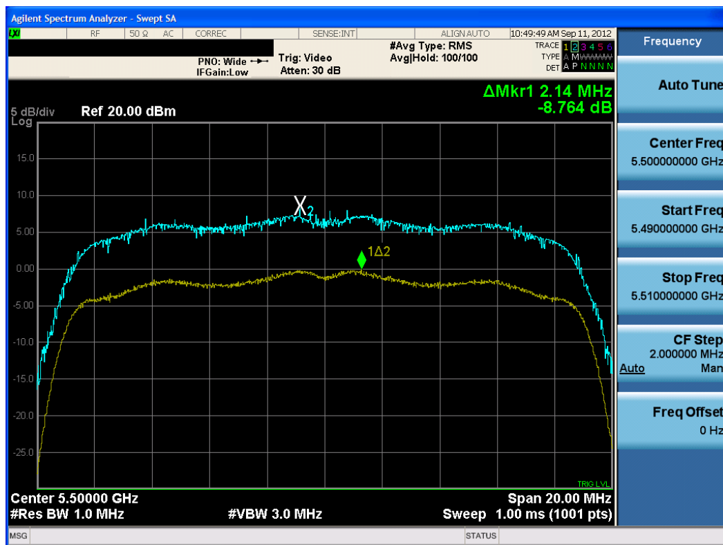
Plot 6-70. Peak Excursion Ratio Plot (20MHz BW 802.11n (UNII Band 3) – Ch. 100)
