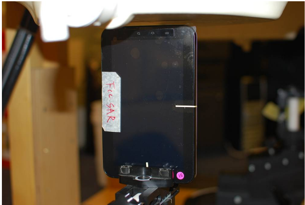
Figure 20-7 SAR Test Setup Photo 6 – Bottom at 0.5 cm
