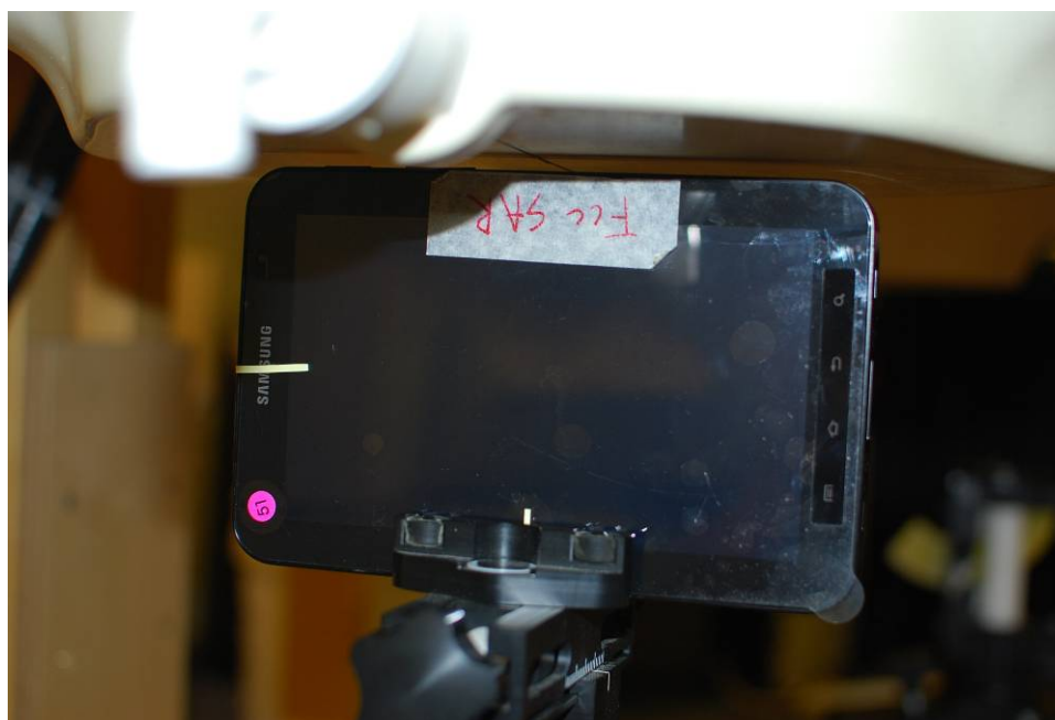
Figure 20-6 SAR Test Setup Photo 5 – Right at 0.5 cm
