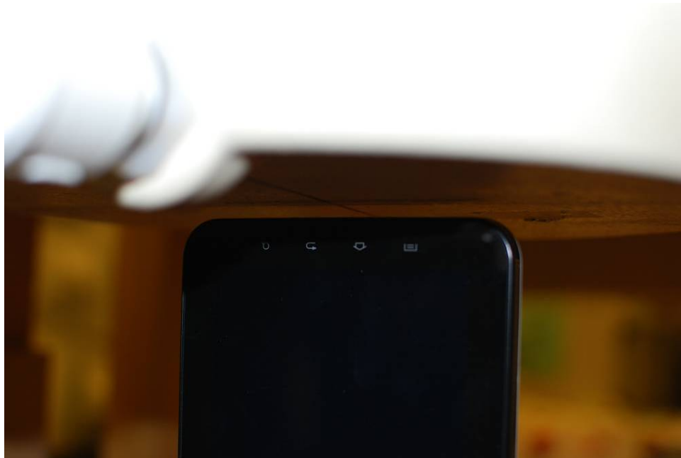
Figure 20-6 SAR Test Setup Photo 6 – Bottom at 0.5 cm
