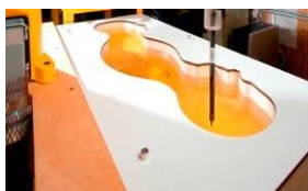
Figure 6-2 SAM Phantom with Simulating Tissue
