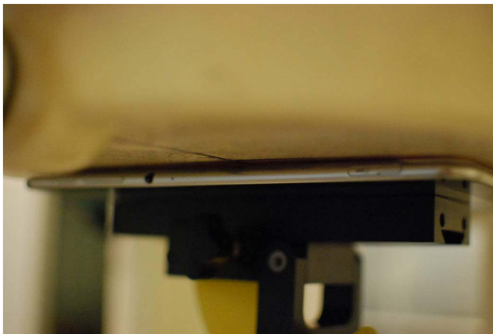
SAR Test Setup Photograph 1 – Back at 0.0 cm
