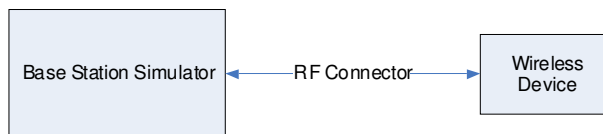
Figure 14-1 Power Measurement Setup
