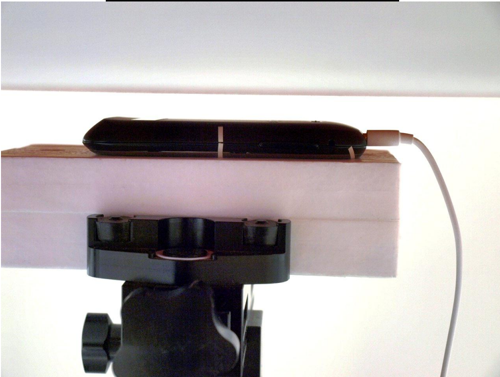
Body Rear w/ 10 mm Separation (w/ Headset)
