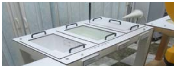
Figure 3.6 Modular Flat Phantom
