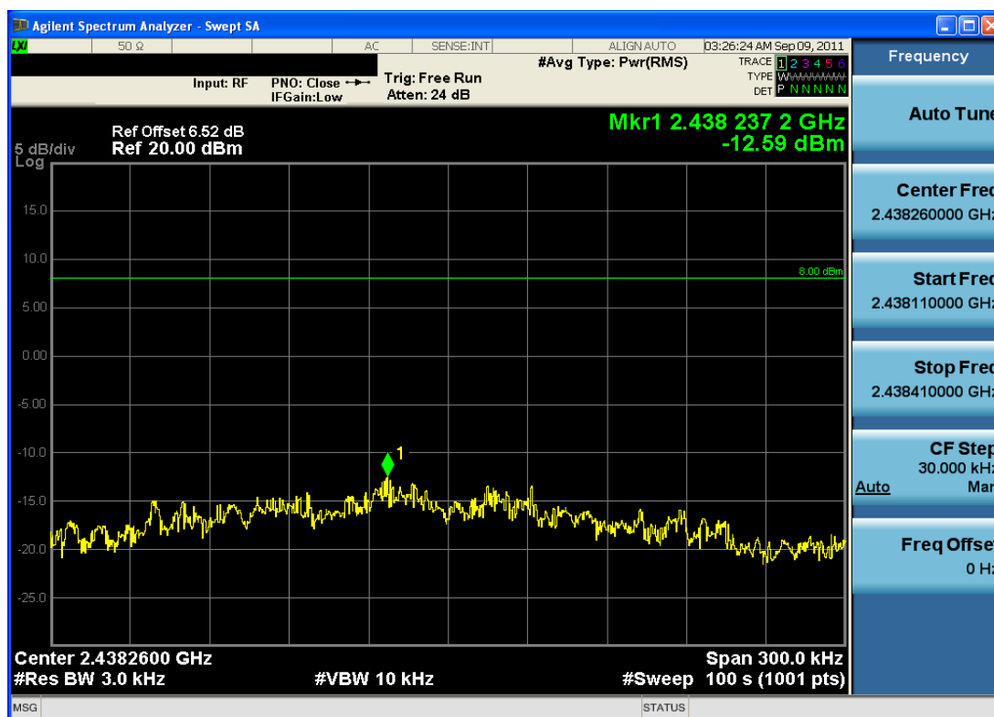
Plot 6-17. Power Spectral Density Plot (802.11n – Ch. 6)
