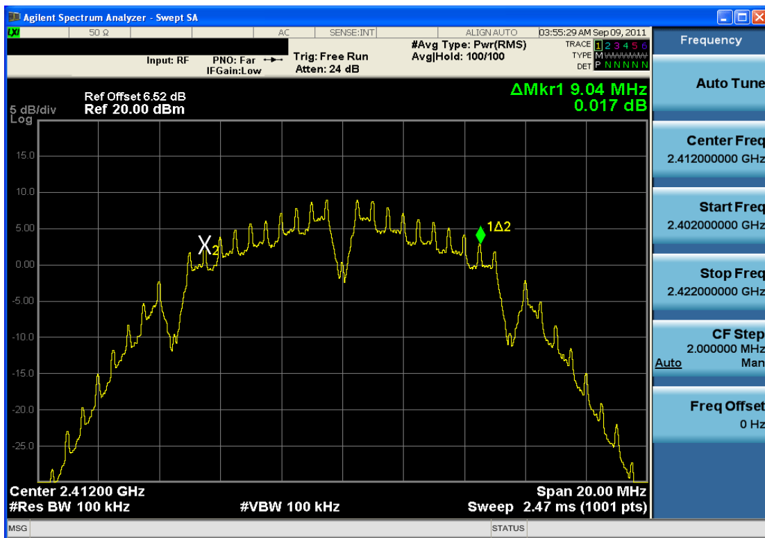
Plot 6-1. 6dB Bandwidth Plot (802.11b – Ch. 1)
