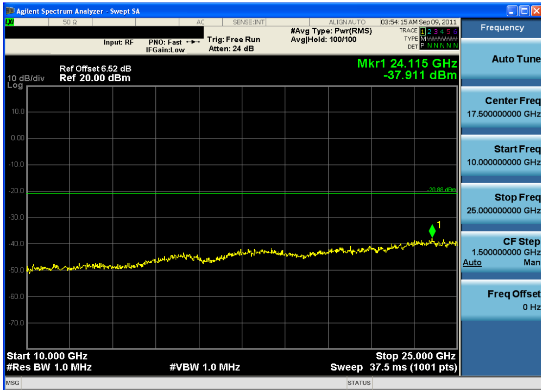
Plot 6-26. Conducted Spurious Plot (802.11b – Ch. 1)
