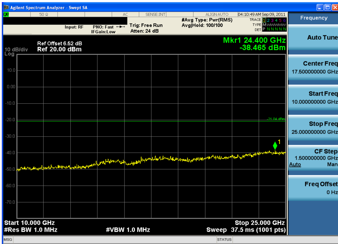
Plot 6-30. Conducted Spurious Plot (802.11b – Ch. 11)
