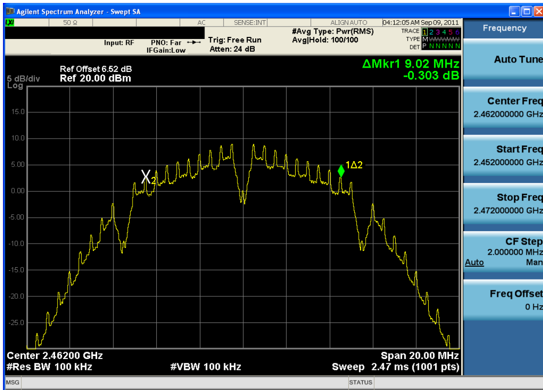
Plot 6-3. 6dB Bandwidth Plot (802.11b – Ch. 11)
