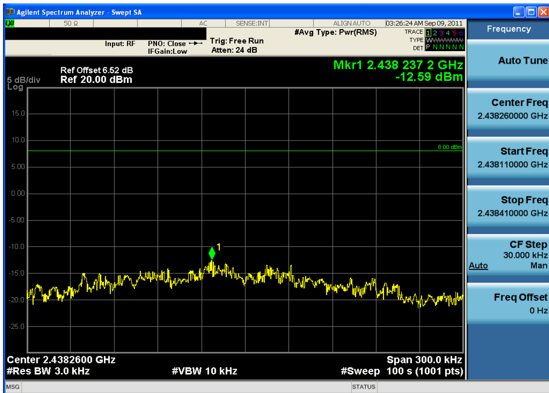
Plot 6-17. Power Spectral Density Plot (802.11n – Ch. 6)
