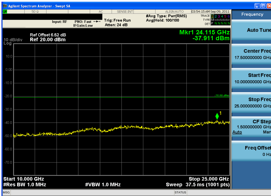
Plot 6-26. Conducted Spurious Plot (802.11b – Ch. 1)
