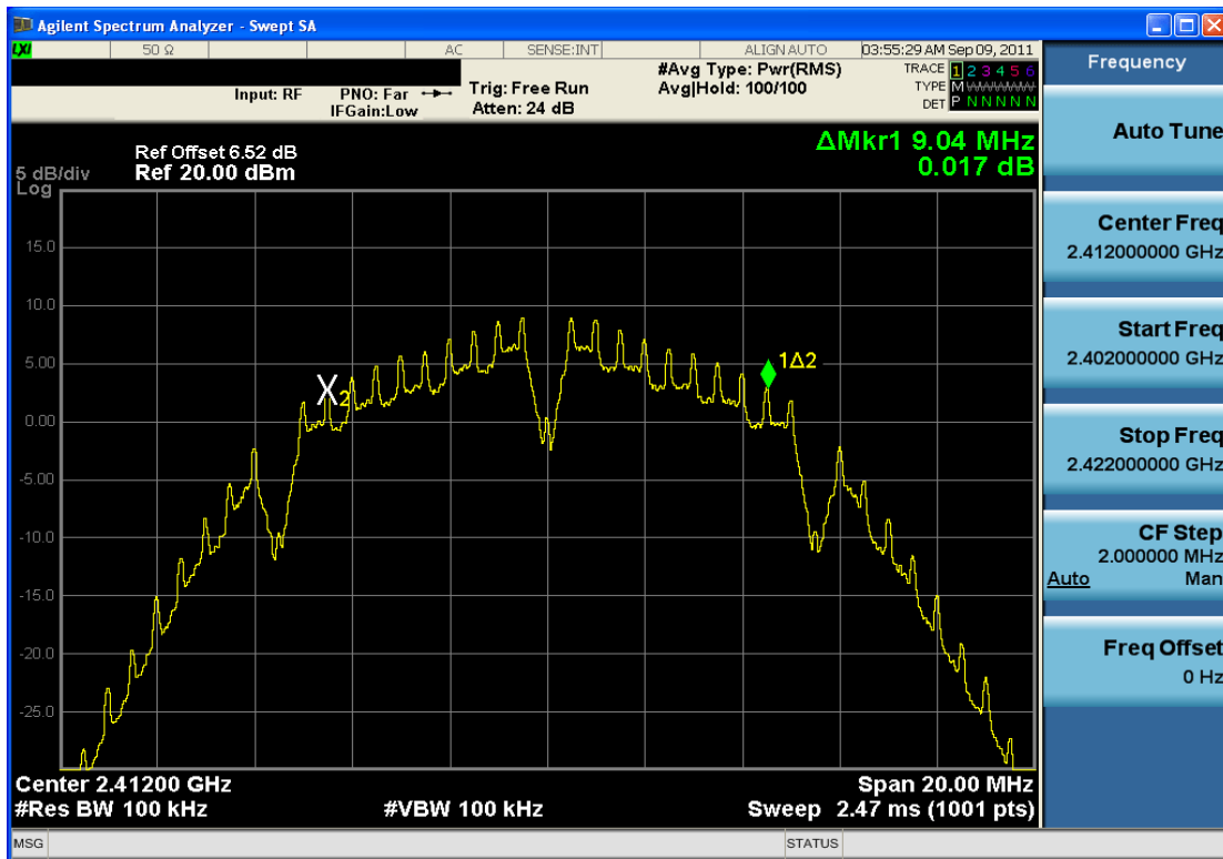
Plot 6-1. 6dB Bandwidth Plot (802.11b – Ch. 1)
