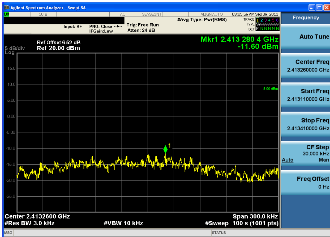
Plot 6-13. Power Spectral Density Plot (802.11g – Ch. 1)
