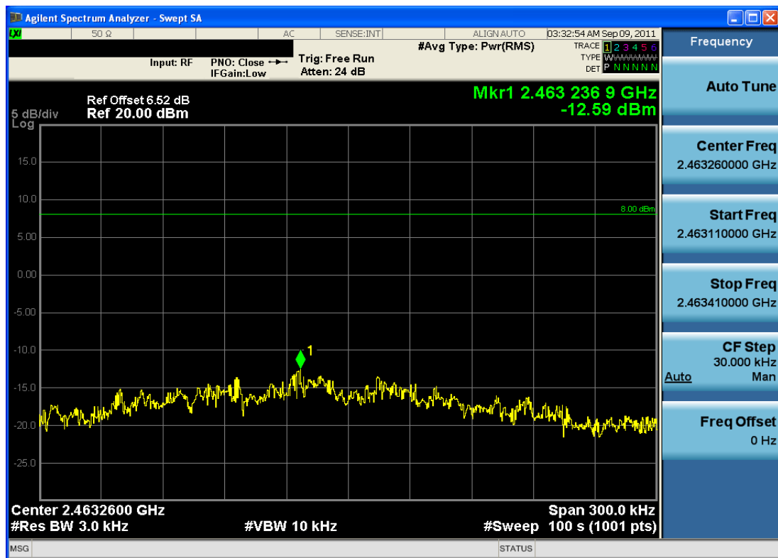
Plot 6-18. Power Spectral Density Plot (802.11n – Ch. 11)
