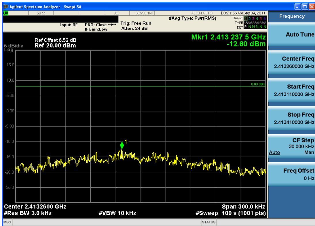
Plot 6-16. Power Spectral Density Plot (802.11n – Ch. 1)
