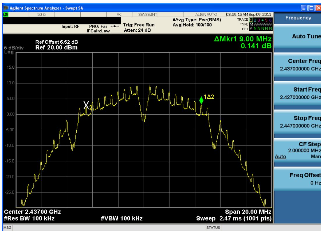
Plot 6-2. 6dB Bandwidth Plot (802.11b – Ch. 6)
