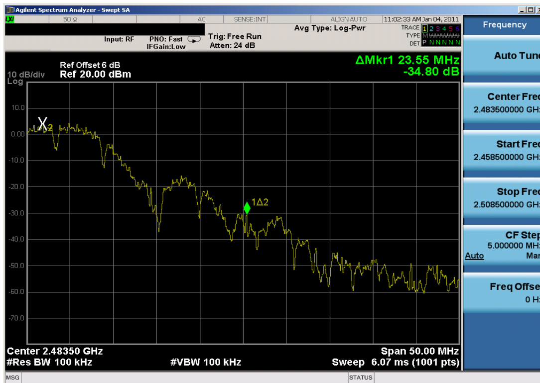
Plot 6-20. Band Edge Plot (802.11b – Ch. 11)
