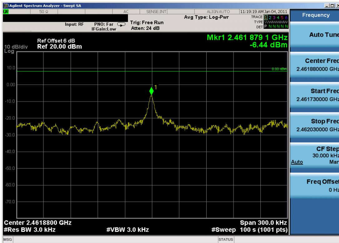
Plot 6-15. Power Spectral Density Plot (802.11g – Ch. 11)
