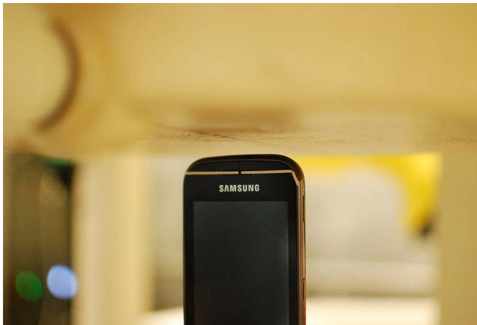
Figure 21-9 SAR Test Setup Photo 9 – Top at 1.0 cm
