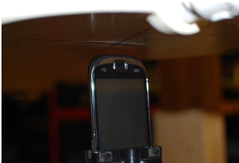
Figure 21-10 SAR Test Setup Photo 10 Body Bottom at 1.0 cm
