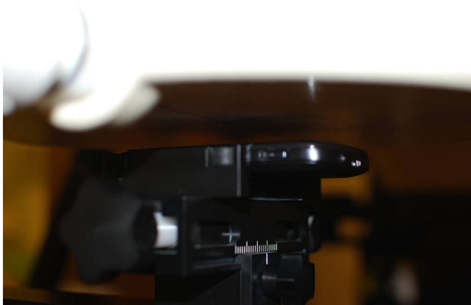
Figure 21-6 SAR Test Setup Photo 6 Body Front at 1.0 cm
