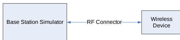
Figure 11-1 Power Measurement Setup
