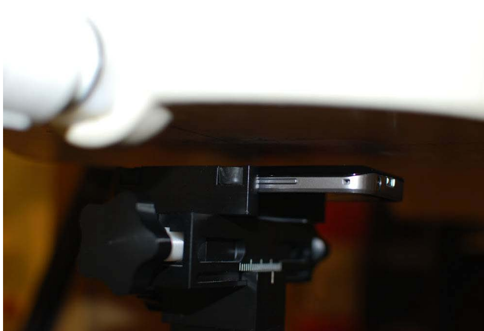
Figure 21-5 SAR Test Setup Photo – Back at 1.0 cm
