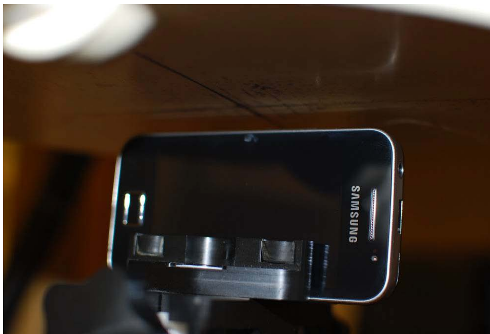
Figure 21-8 SAR Test Setup Photo – Left at 1.0 cm
