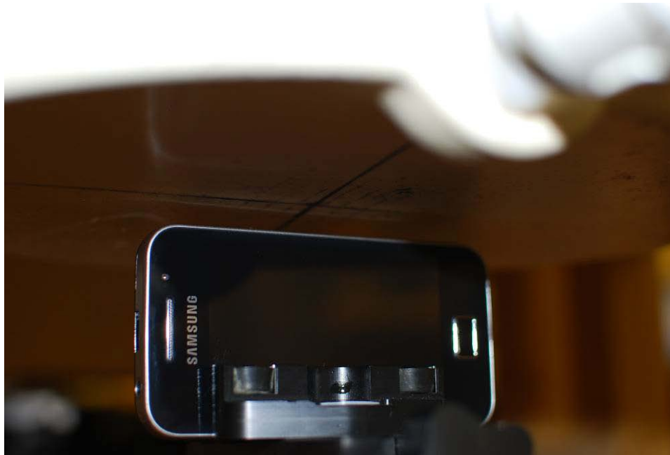
Figure 21-7 SAR Test Setup Photo - Right at 1.0 cm
