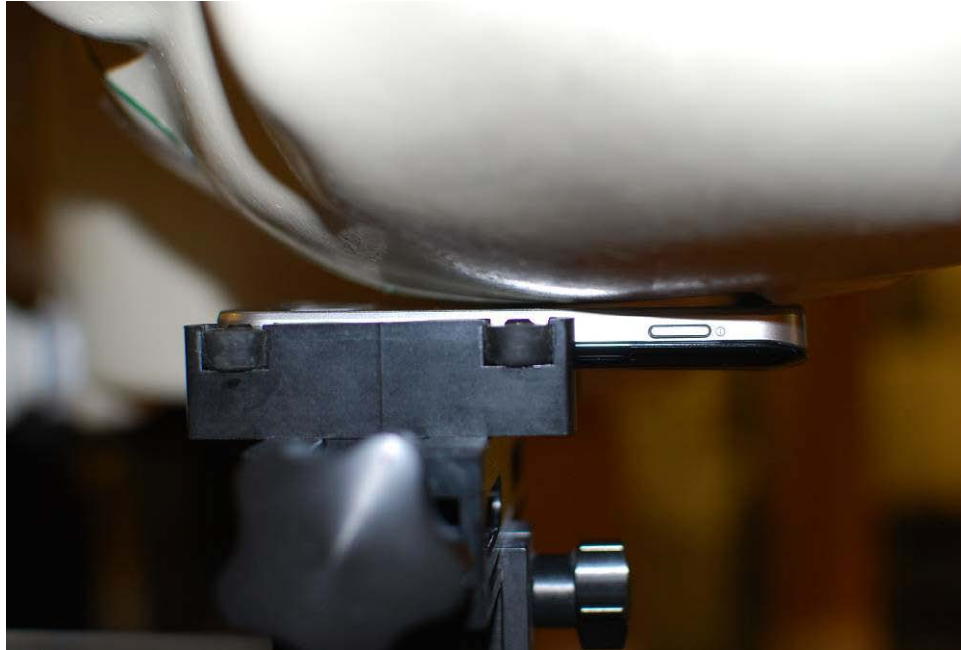
Figure 21-3 SAR Test Setup Photo – Left Touch
