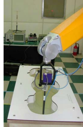
Figure 3.2 Photograph of the probe and the Phantom
