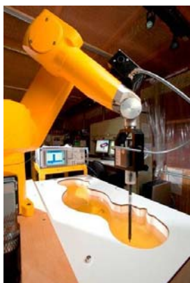
Figure 3-1 SAR Measurement System
