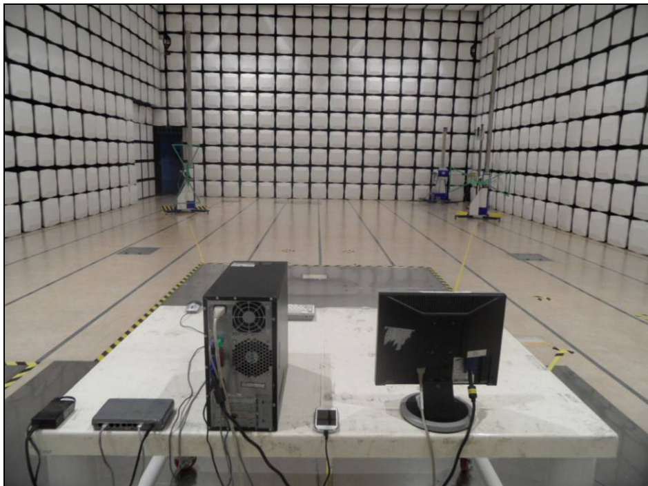
[ Radiated Disturbance for Below 1 GHz – Rear ]
