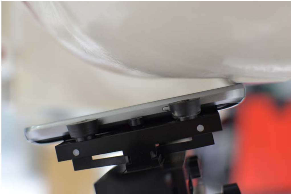
SAR Test Setup Photo 4 – Left Tilt
