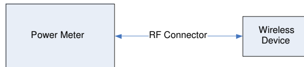
Figure 15-1 Power Measurement Setup
