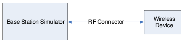
Figure 14-1 Power Measurement Setup
