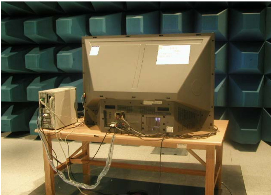
Picture 4. Radiated Emission (Rear)
