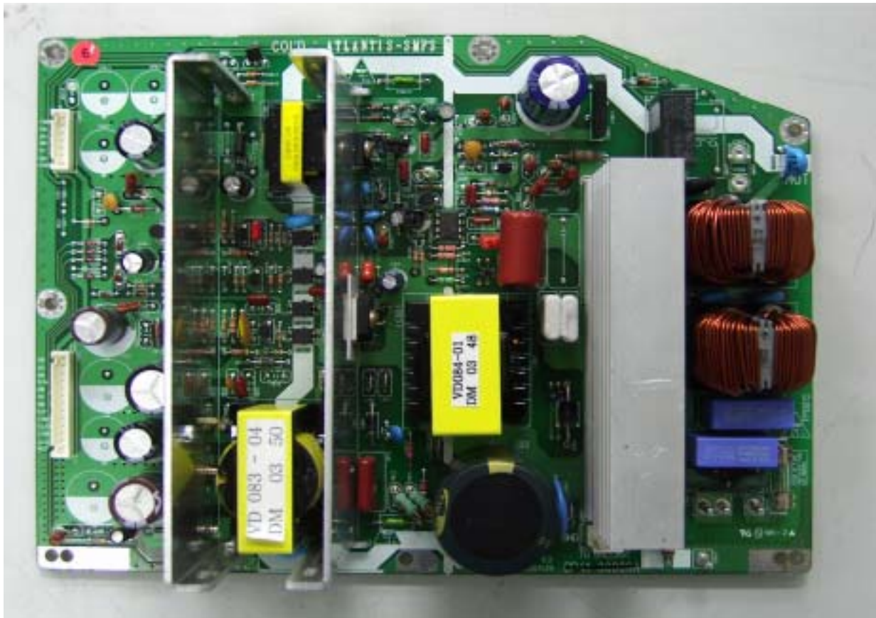
SMPS board top view
