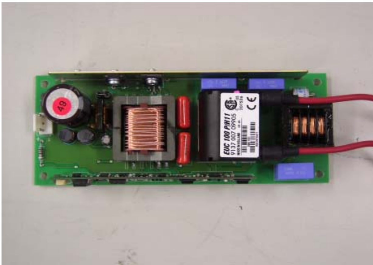
Ballast board top view
