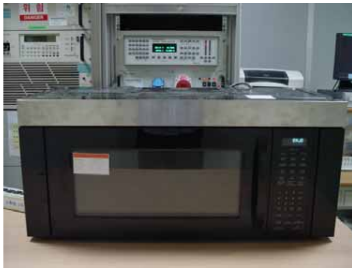
Fig.3 Test Setup for RF output power
