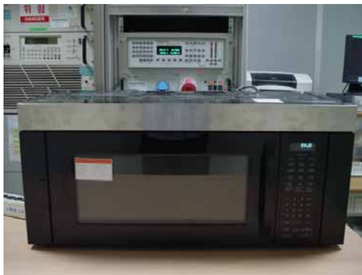
Fig. 2 Test Setup for Input power
