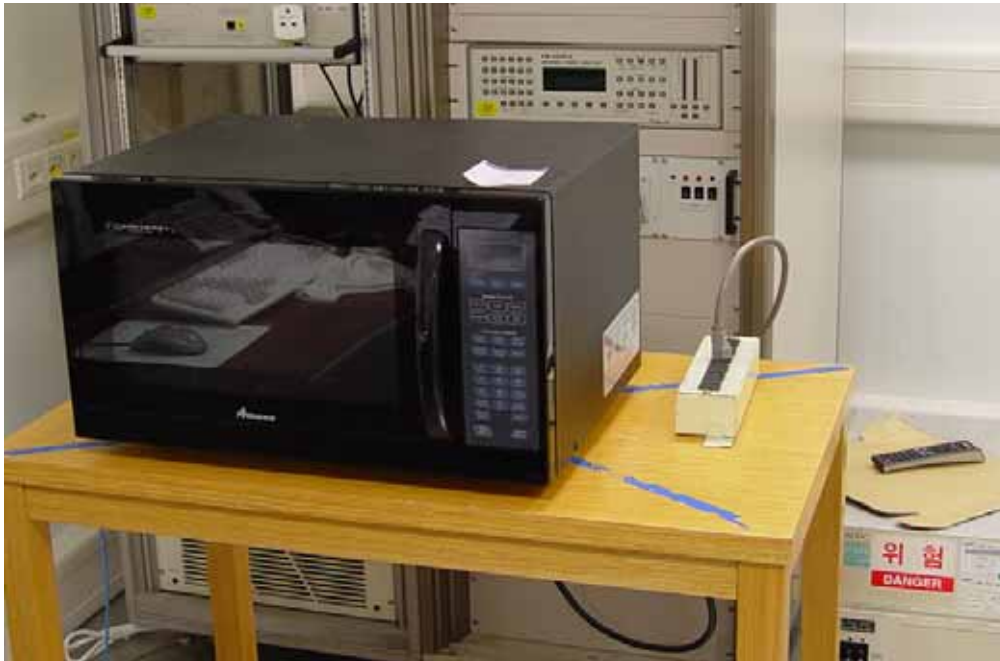
Fig. 2 Test Setup for Input power
