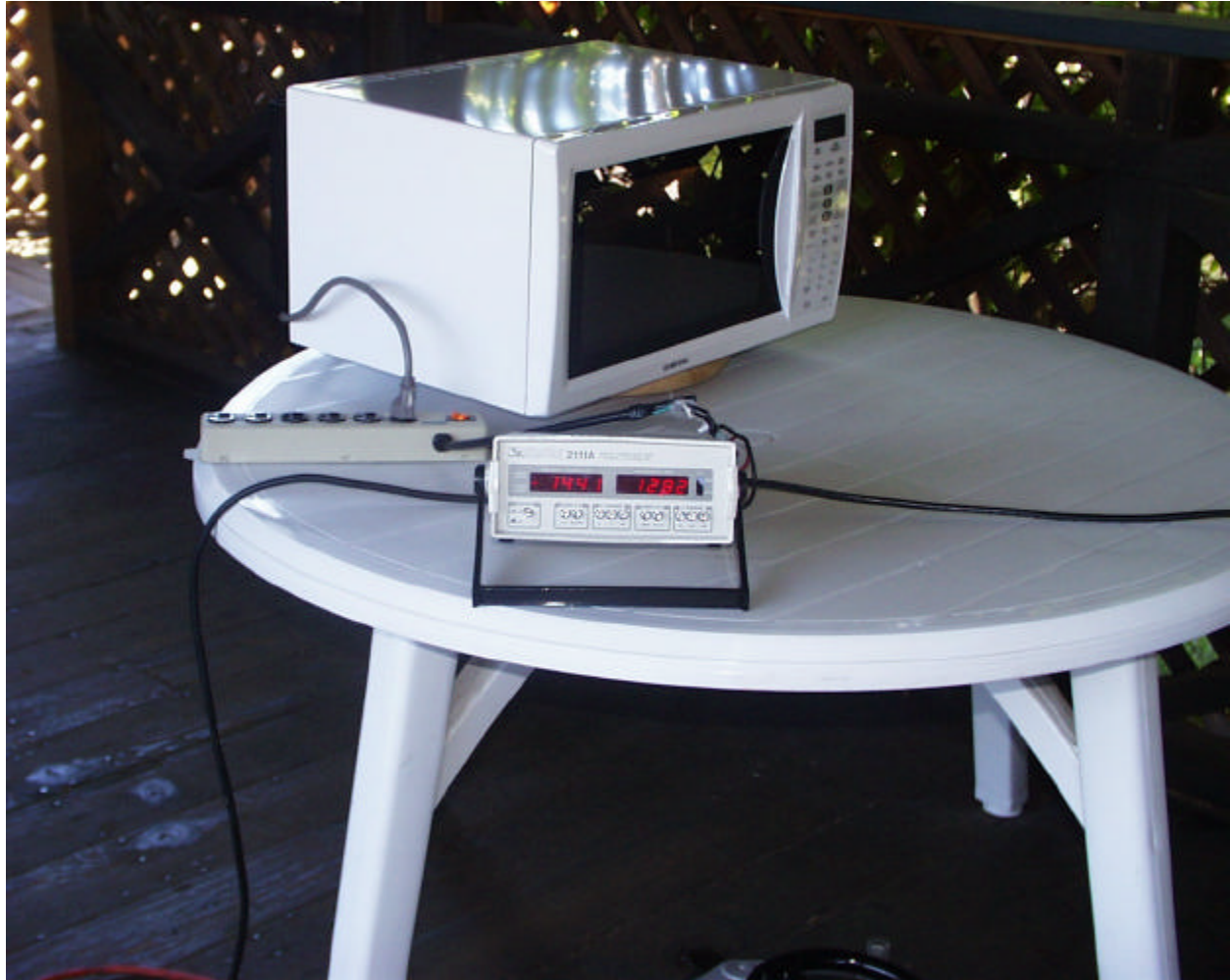
Input Power Test Setup
