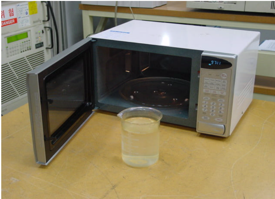
Fig.3 Test Setup for RF output power
