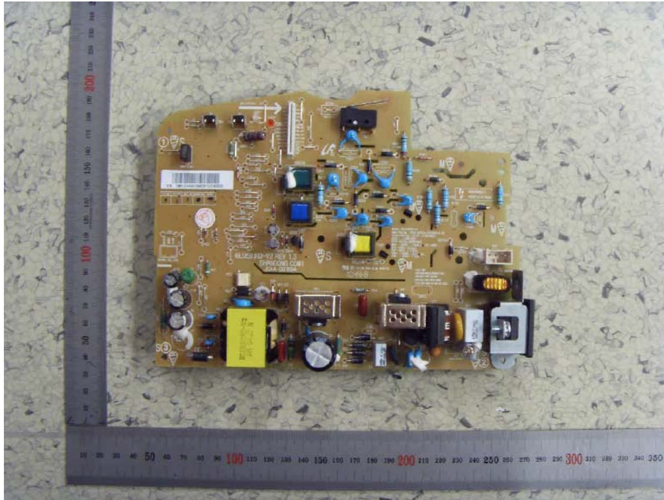
SPTH, Bluebird_V2 (ML-1670_SMPS PBA_Top Side)
