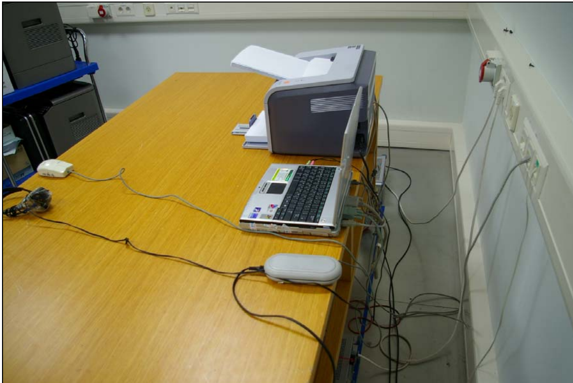
Picture 2. Conducted emission (Rear)
