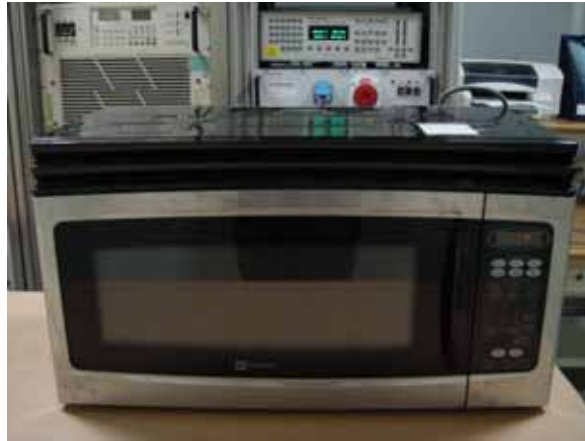
Fig.3 Test Setup for RF output power
