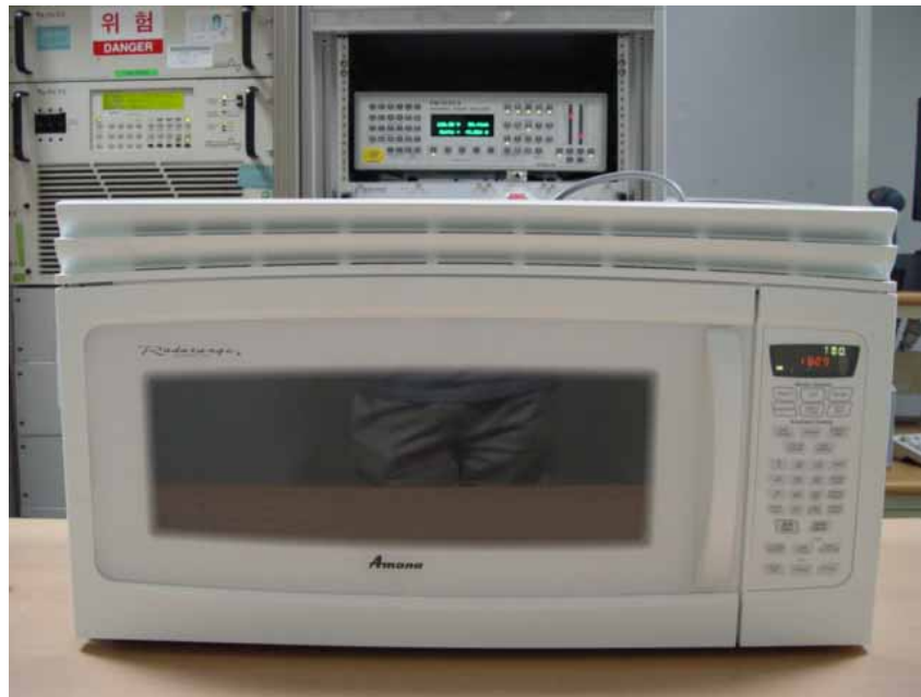
Fig. 2 Test Setup for Input power
