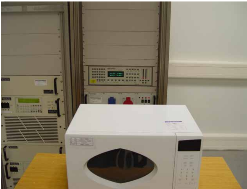
Fig. 2 Test Setup for Input power
