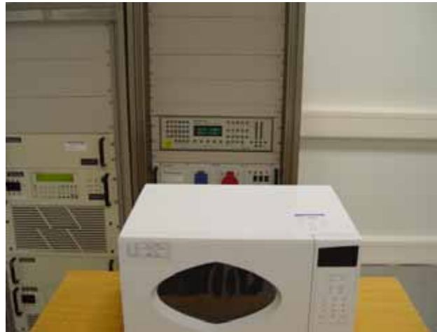
Fig.3 Test Setup for RF output power
