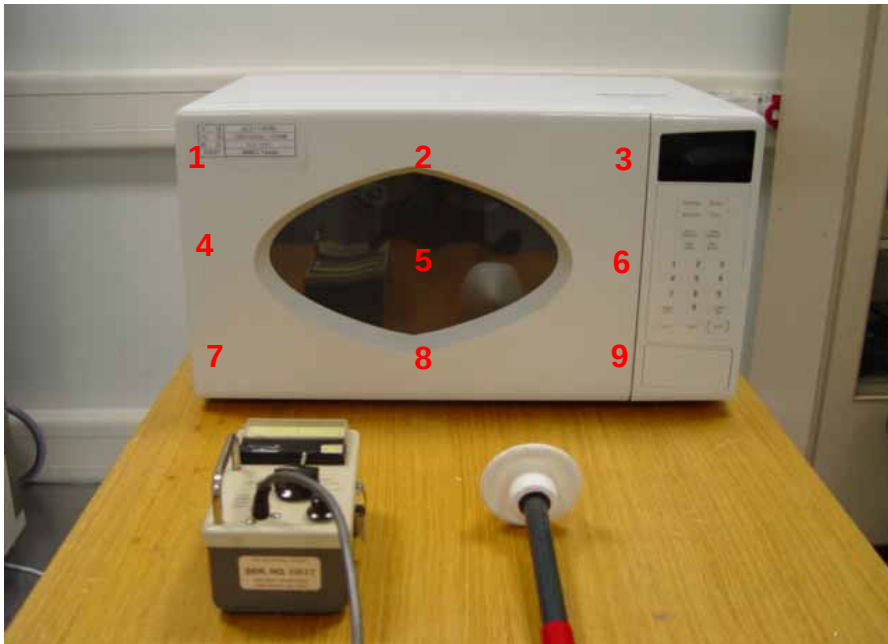
Fig. 1 Test Setup for Radiation Hazard Measurement
