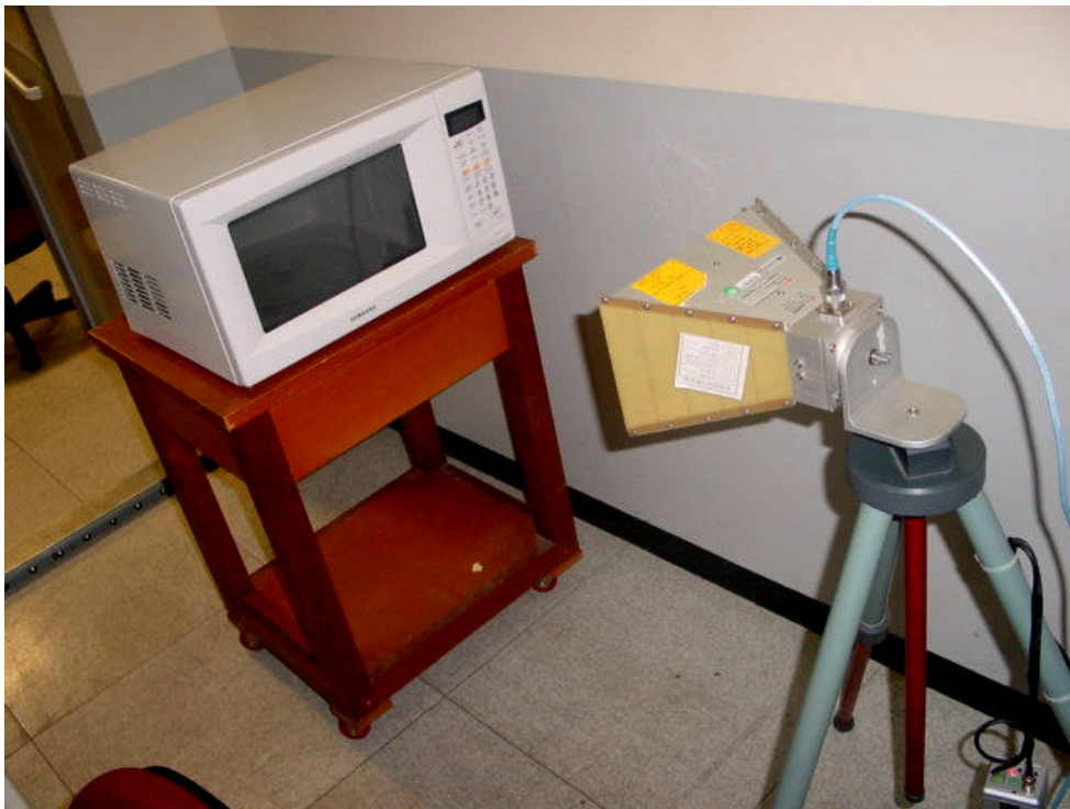
Fig. 4 Operating Frequency Measurements Configuration
