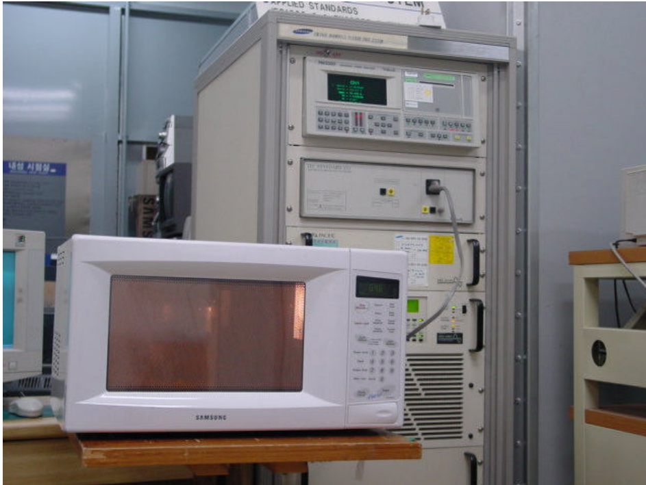
Fig. 2 Test Setup for Input power
