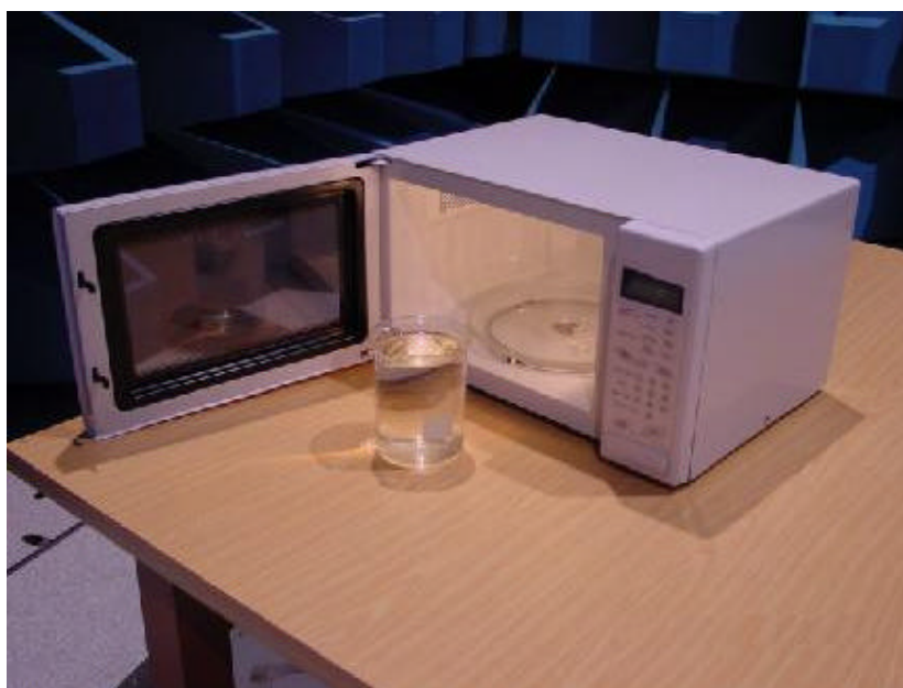
Fig.3 Test Setup for RF output power
