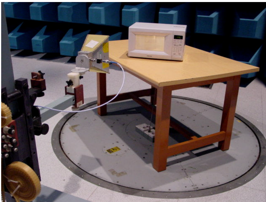
Fig. 9 Radiated Emission setup(1 - 25GHz)
